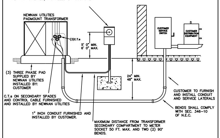
UNDERGROUND COMMERCIAL 3Ø TRANSFORMER RATED METER INSTALLATION WITH ONLY ONE CUSTOMER
