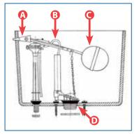
A The flushing arm and lift chain are not working properly.
